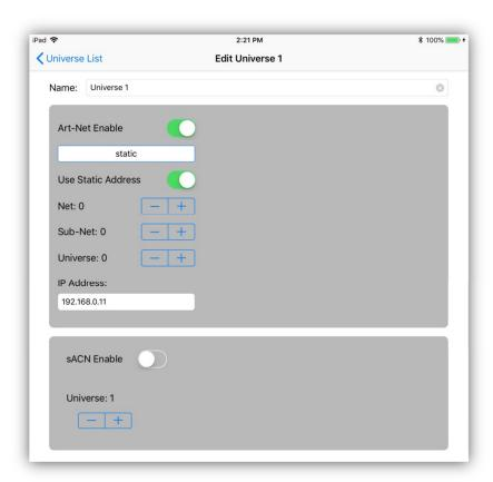
You can configure the Art-Net universe to use a static IP address or have the app search for Art-Net nodes on the network. Using a static address can be more reliable in that the node, if set correctly, will most likely be at a known location on the network. To use a static IP address, turn on the "Use Static" switch and then enter the correct IP address for the Art-Net node.
