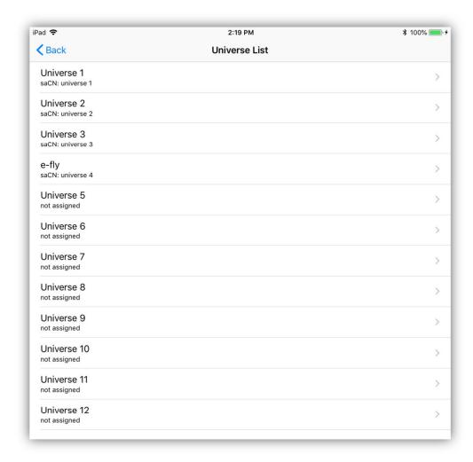
This app can support up to twelve DMX512 universes. If you are using a single 4 Cast DMX Bridge that's making its own network, then you will only be concerned with the first four. If you need additional universes, you will have to connect additional 4 Cast DMX Bridges or other nodes using an external network. This app only requires that you use at least one 4 Cast Bridge. Additional nodes can use other products by any manufacturer.
