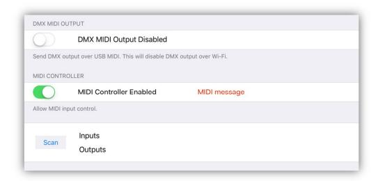
The DMX MIDI Output switch enables a wired connection between your IPad and the 4 Cast DMX Bridge. Instead of sending DMX packets over Wi-Fi, it will send them over USB using MIDI messages. The Wi-Fi messages will be turned off as the wired connection will replace it. This can be helpful when radio or network interference makes it difficult to connect to the bridge. Only universes 1-4 are supported. See the MIDI chapter for details.
